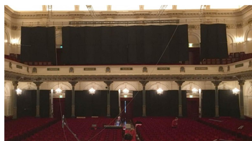
Figure 13. Concertgebouw Amsterdam: test setup with curtains below and above rear balcony.
