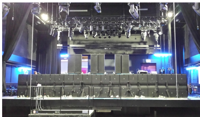
Figure 9 – Measurement set up on the stage of the large pop hall with 18 subwoofers and 6 arrays
