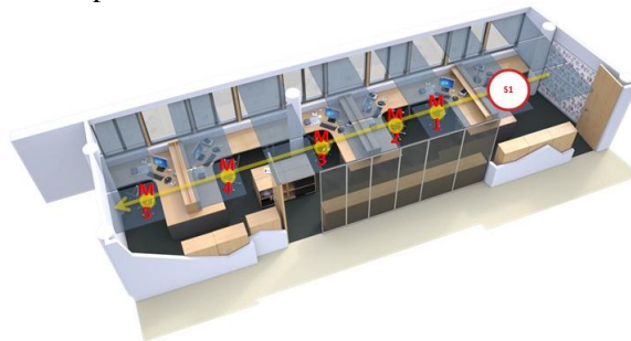
Illustration 2: Path “a”: Source in S1 (workstation located on the right), measurement path from right to left.
