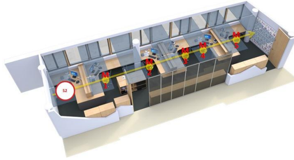
Illustration 3: Path “b”: Source in S2 (workstation located on the left), measurement path from left to right.
