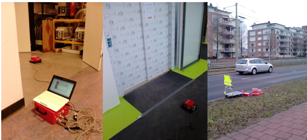
f3.1 Near field vibration measurements next to compressor (left), elevator (middle) and traffic (right)
