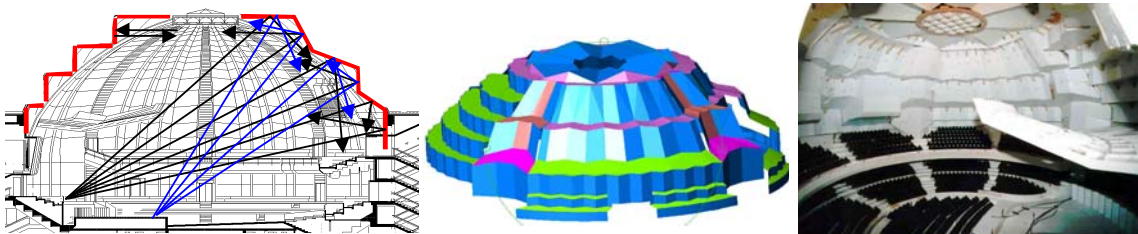
FIGURE 11. Renovation concept of the Tonhalle Düsseldorf. Left: section with geometrical reflection paths; middle: 3D visualization of the reflector geometry; right: photo of the scale model 1:12.
