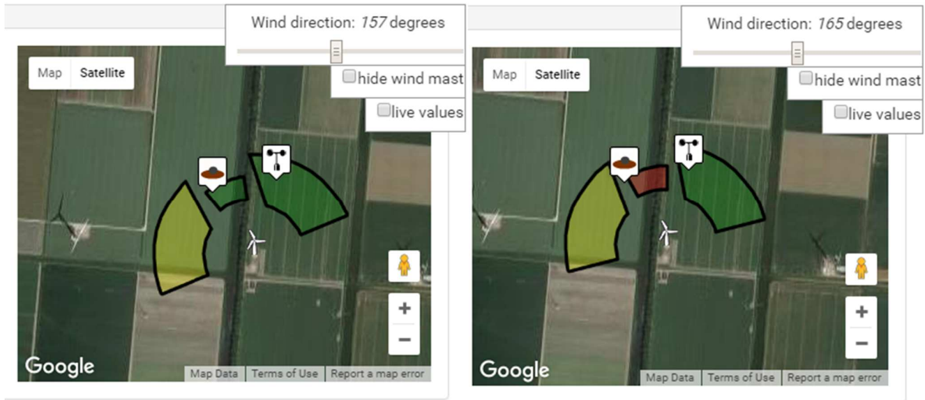
Figure 4 current measurement positions and their allowable range. (left: all valid, right: microphone position not valid)
