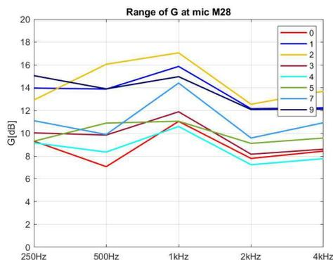
**Figure 7a.** Measured balance of G 2017 at the alto violin position
