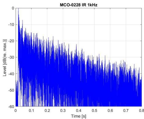
**Figure 6b.** Measured impulse response from trumpets to alto violins 2020 with increased strength of reflections.
