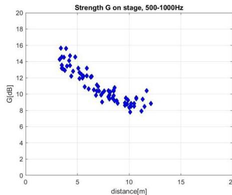
**Figure 9a.** Measured strength G 2017 vs distance at the stage
