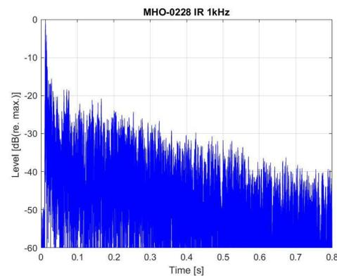
**Figure 6a.** Measured impulse response from trumpets to alto violins 2017 with very low strength of reflections.
