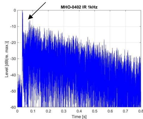
**Figure 5a.** Measured impulse response from 1st violins to trumpets 2017 with missing early reflections
