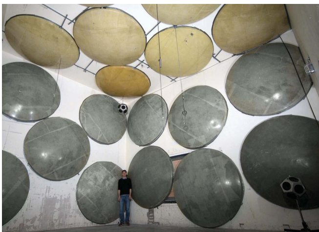
Figure 1. Reverberation room at Peutz with circular diffusers
