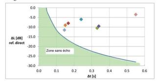
Figure 1. Identification of echoes before refurbishment
