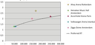
**Figure 15**. Average RT in empty hall as function of volume for the halls presented in this paper. The preferred RT refers to Eq. (1).
