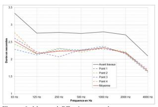
**Figure 6.** Measured RT<sub>30</sub> in unseated, concert set-up before (black line) and after (red line, average) refurbishment
