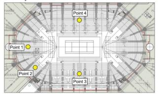
Figure 5. RT<sub>30</sub> measurement locations after completion
