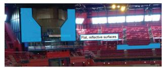
Figure 2. Reflecting surfaces causing adverse echoes
