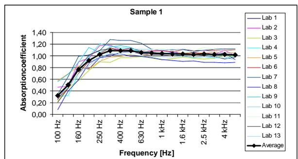
Figure 1: Measurement results of the sound absorption in 13 labs. The black solid line gives the average result.
