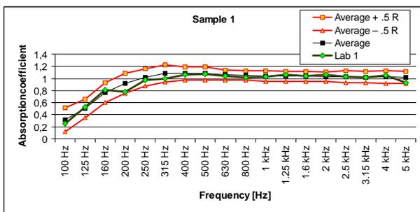
Figure 6: Illustration of the average and spread ( $\pm 1/2R$ ) of sample 1 and the individual result of one laboratory (green).
