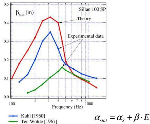
Figure 4: The edge effect: the absorption of a finite sample is composed of the absorption of an infinite sample ( $\alpha_s$ ) and a factor  $\beta$  multiplied with the relative edge length E. The graph show the  $\beta$  from experimental and theoretical studies [5].
