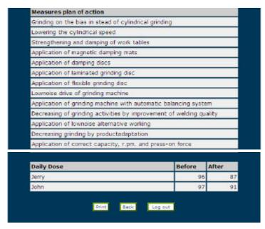
Figure 4. Example of calculated effect of specified sound reducing measures.
