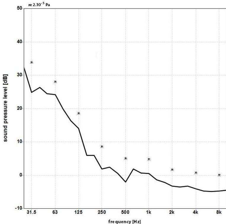
The background noise level of the ventilation system in the unoccupied hall can be compared with the threshold of hearing (cf. ISO 8253-2:2009), both are given in octave bands in the next graph (measurement (black line), threshold (red)).
