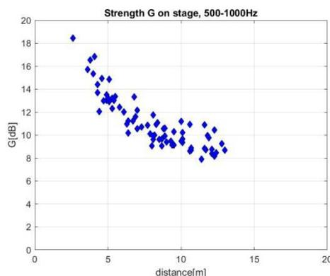
**Figure 9a.** Measured strength G 2017 vs distance at the stage
