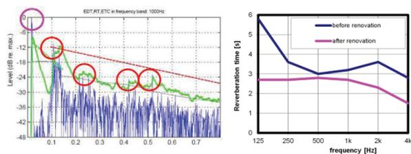
**Figure 8.** Ahoy arena, Rotterdam, Left: Impulse response before renovation. Purple circle is direct sound, red circles indicate too strong reflections. Right: reverberation times before and after renovation.
