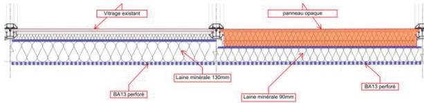
Figure 3. Low frequency absorbers on attic level
