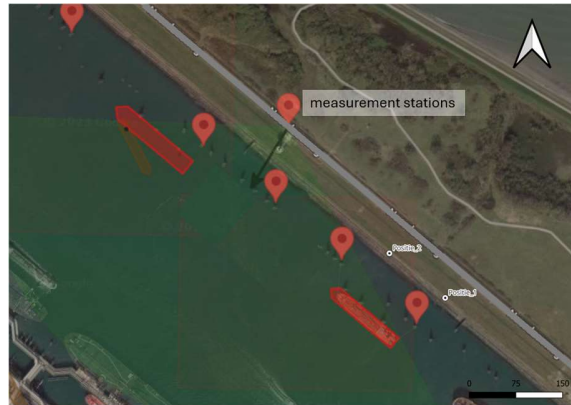
Figure 6: Measurement network to automatically determine the sound power level of moored sea vessels.
